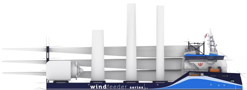
Picture 6. Design of an offshore wind feeder vessel (source: C-Job.com)
